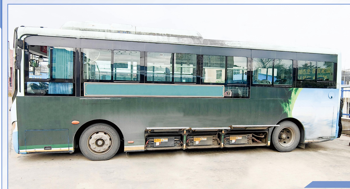
Bus battery exchange 537.6V 105Ah 6m EV bus
